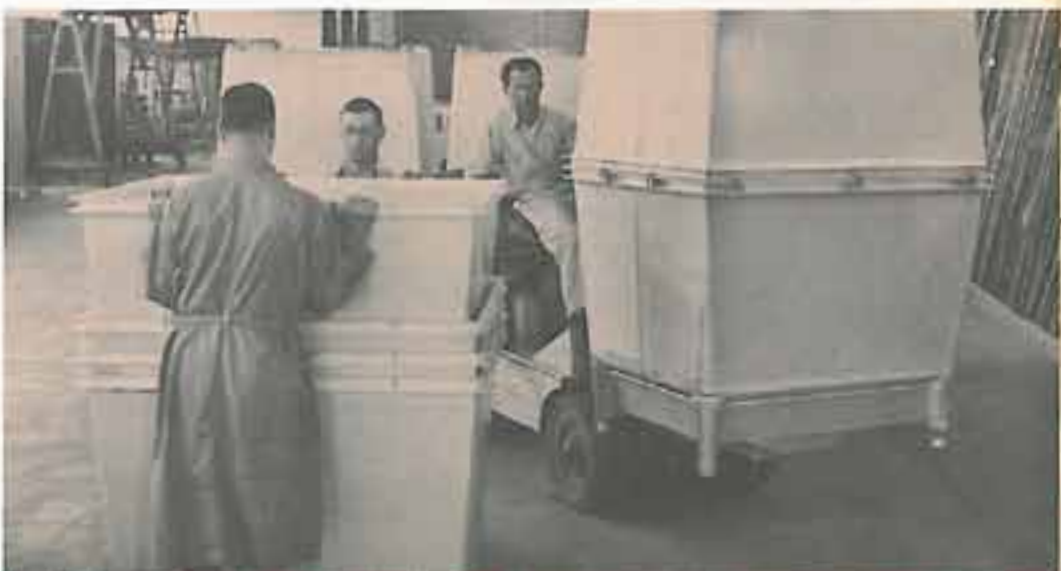
Below: Bulk sugar bins are used by food manufacturers to transport refined sugar in bulk form to their own plants. Each bin holds 1,000 pounds and protects the sugar against all temperature and weather conditions.
