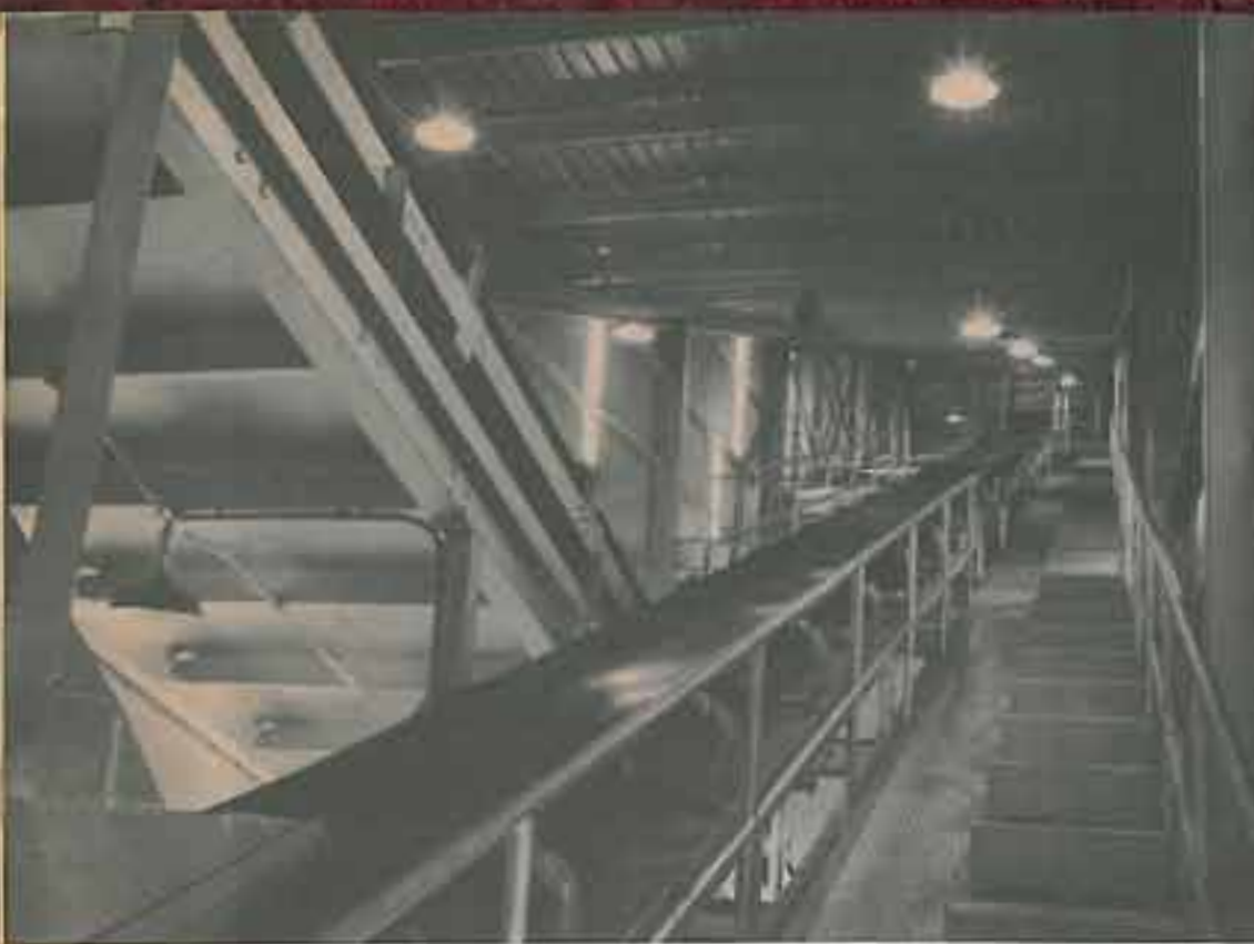
Throughout the refining process, sugar is moved and handled automatically, never touched by hand. This conveyor belt, which moves raw sugar into the vast warehouse, is typical of the completely automatic equipment found in all units of the refinery.
