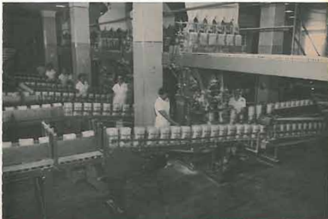
Packing plant employees watch closely to see that bags are filled, weighed and sealed properly. This view shows funnel-like equipment (near the ceiling) through which refined sugar flows from storage bins to packaging machines.
