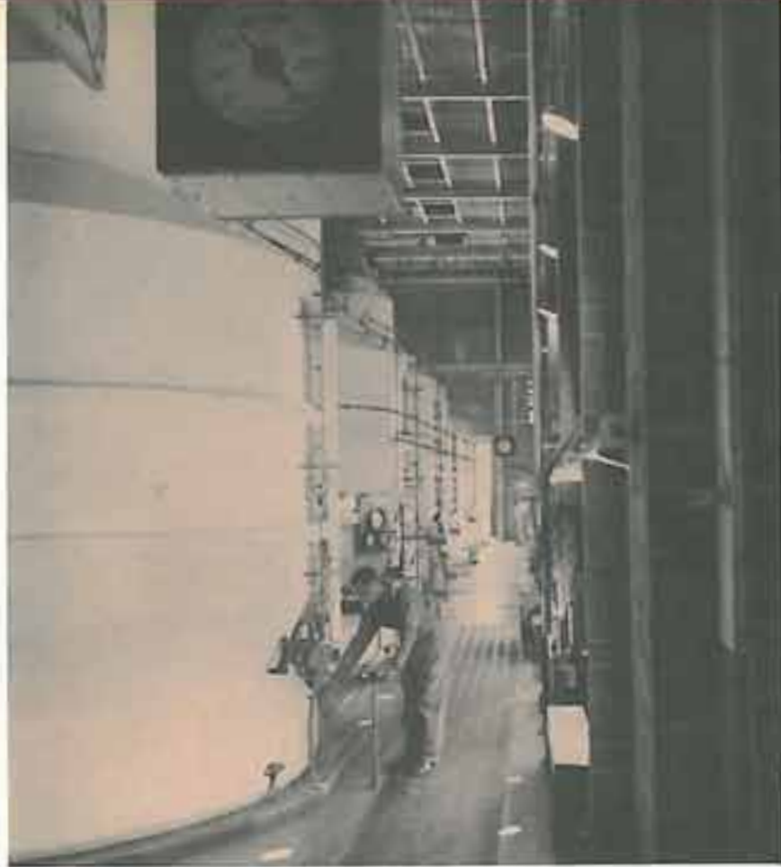
This section of the Imperial refinery, with its row of big vacuum pans, is called a "pan floor". Here both white sugar and brown sugar, in liquid form, are boiled to the crystallization point.
